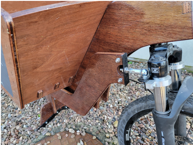
Steering bar and bracket
